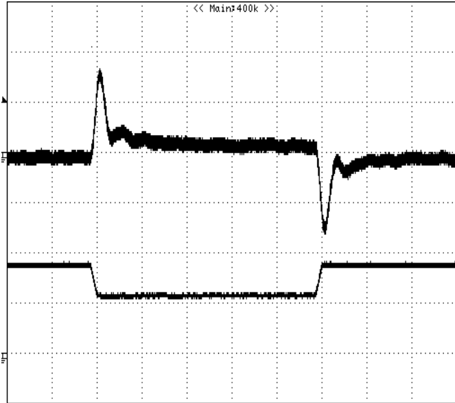
Figure 8: Output voltage response to step-change in load current (75%-50%-75% of I_o , max; di/dt = 0.1A/\mu s ). Load cap: 10\mu F , tantalum capacitor and 1\mu F ceramic capacitor. Top Trace: V_{out} (100mV/div, 200us/div), Bottom Trace: I_{out} (5A/div). Scope measurement should be made using a BNC cable (length shorter than 20 inches). Position the load between 51 mm to 76 mm (2 inches to 3 inches) from the module
