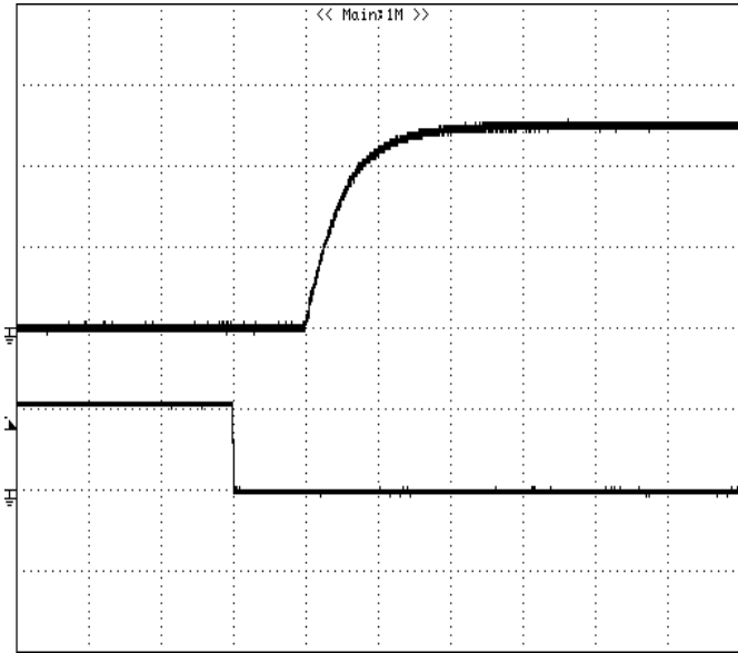
Figure 4: Turn-on transient at full rated load current (CC Mode load ) (5 ms/div). V_{in}=48V . Top Trace: V_{out} , 2V/div; Bottom Trace: ON/OFF input, 5V/div
