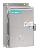
Non-reversing NEMA contactor, Size 0, Single phase full voltage, Contactor amp rating 18A, 3 wire (NO aux included), 110V 50Hz / 120V 60Hz coil, Non-combination type, Encl NEMA type 4X 304 S-Steel, Water/dust tight noncorrosive, Standard width enclosure
