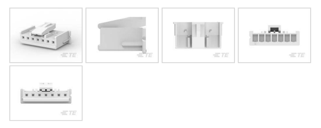
Connector Product Type: Housing Connector & Housing Type: Receptacle Connector System: Wire-to-Board Number of Positions: 7 Centerline (Pitch): 2.5 mm [.098 in ]
