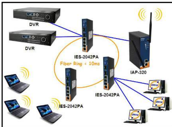
Connections of redundancy
