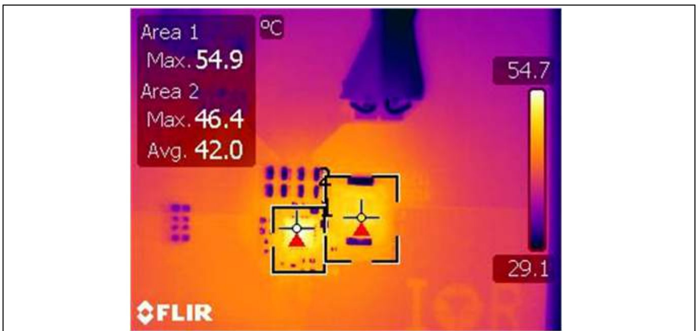
Figure 24 Thermal Image of the board at 3 A load IR3883 = 55 °C, L= 46 °C, Amb = 25 °C
