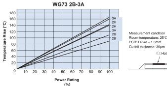
Regarding the temperature rise, the value of the temperature varies per conditions and board for use since the temperature is measured under our measuring conditions.
