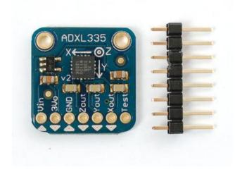
The ADXL335 can measure at least +/- 3G in the X, Y and Z axis. It is perfect for high-resolution static acceleration measurements such as tilt-sensing, as well as for moderate dynamic accelerations from motion, shock or vibration.
