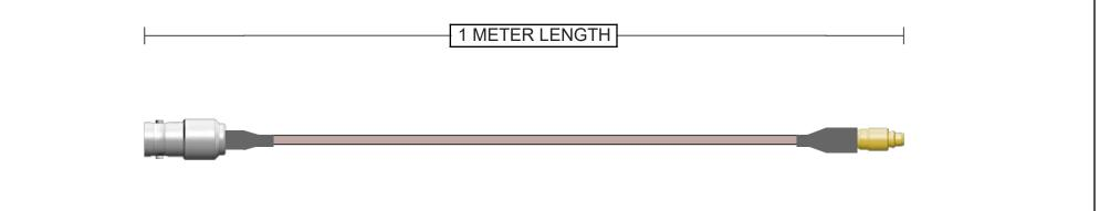
Connector A 112631 BNC Jack Straight Brass Nickel + Heatshrink 50 Ohm RG-178 Continuity/Hi-Pot Connector B 262100 MMCX Plug Straight Brass Gold + Heatshrink
