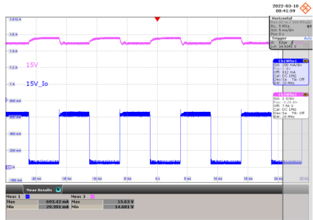
Figure 20 – 400 VDC Input. CH1: I OUT , 200 mA / div., 5 ms / div. CH3: V OUT , 2 V / div., 5 ms / div. V OUT (MAX) = 15.63 V, V OUT (MIN) = 14.681 V.
