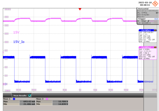
Figure 16 – 60 VDC Input. CH1: I OUT , 200 mA / div., 5 ms / div. CH3: V OUT , 2 V / div., 5 ms / div. V OUT (MAX) = 15.709 V, V OUT (MIN) = 14.839 V.
