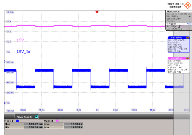
Figure 32 – 60 VDC Input. CH1: I OUT , 200 mA / div., 5 ms / div. CH3: V OUT , 2 V / div., 5 ms / div. V OUT (MAX) = 15.314 V, V OUT (MIN) = 14.839 V.
