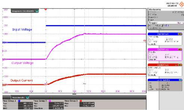
Figure 111 – 400 VDC Input. CR Full Load. CH1: V_{INPUT} , 200 V / div., 4 ms / div. CH3: V_{OUT} , 5 V / div., 4 ms / div. CH4: I_{OUT} , 500 mA / div., 4 ms / div. Rise Time V_{OUT} = 7.449 ms.
