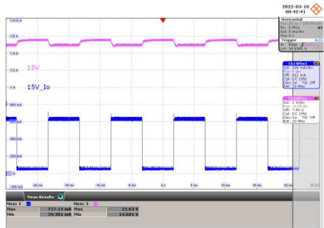
Figure 22 – 550 VDC Input. CH1: I OUT , 200 mA / div., 5 ms / div. CH3: V OUT , 2 V / div., 5 ms / div. V OUT (MAX) = 15.63 V, V OUT (MIN) = 14.681 V.
