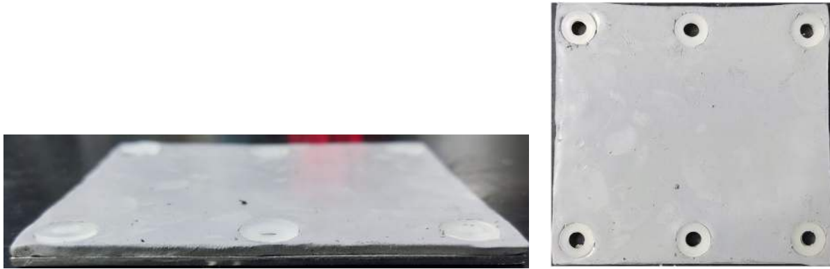
Figure 212 – Assembled Aluminum Sheet, Thermal Pad, and spacer.
