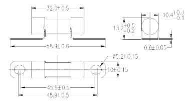
Note: recommend tightening torque is 3.5-4 Nm for M5 screw
