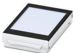
DIN rail housing for use in distribution boards in accordance with DIN 43880, Latching cover (non-detachable), integrated capacitive 2.4" touch display, resolution: 320 x 240 Pixel(s), interface: 4-wire SPI, width: 71.6 mm, height: 45 mm, depth: 13.5 mm, color: light grey (7035)
