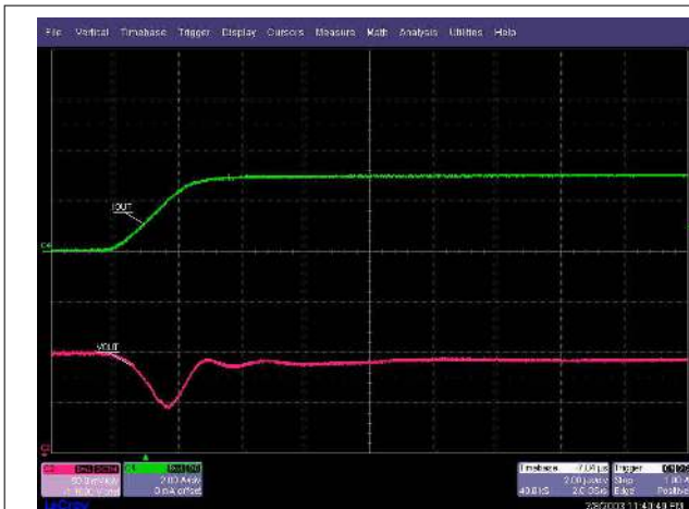
Figure 2-3. TPS7A53EVM-080 Load Transient Results: 1-mA to 3-A Load Step
