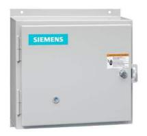
Non-reversing motor starter, Size 1, Three phase full voltage, Solid-state overload relay, OLRelay amp range 0.75-3.4a, 240V 50HZ / 277V 60HZ coil, Non-combination type, Enclosure type 12, Dust/drip proof for indoors, Standard width enclosure
