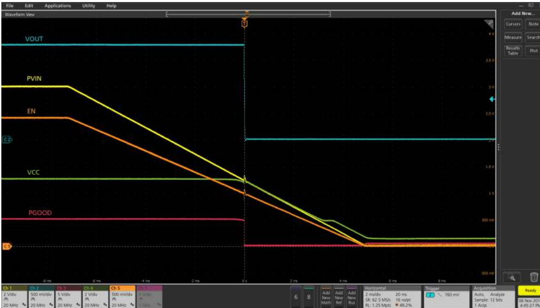
Figure 5 Shutdown with Enable de-assertion at 6A load (Ch1:PV IN , Ch2: V OUT , Ch3: PG, Ch4:V CC , Ch5: Enable)
