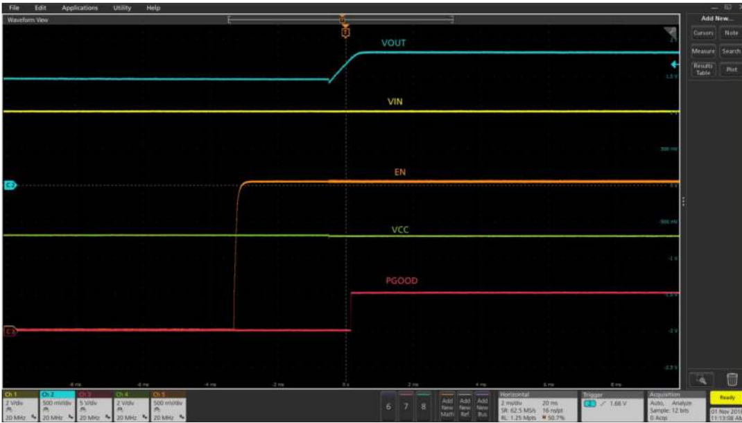
Figure 7 Startup into pre-bias (Ch1:PV IN , Ch2: V OUT , Ch3: PG, Ch4:V CC , Ch5: Enable)
