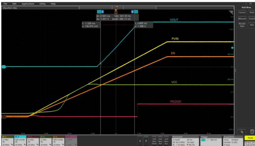
Figure 4 Startup with 6A load (Ch1: PV_{IN} , Ch2: V_{OUT} , Ch3: PG, Ch4: V_{CC} , Ch5: Enable)
