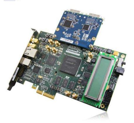
The Cyclone V GX Video Development System is an ideal video processing platform for high-performance, cost-effective video applications. With PCIe x4 lanes and high-speed 3.125 Gbps transceiver capabilities, the Cyclone V GX kit allows for a myriad of functionalities such as prototyping, power measurement, and high-speed communication. Memory interfaces include flash memory, SRAM, and DDR3, creating a complete integrated memory interface solution for memory-intensive applications.
