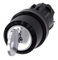
RONIS key-operated switch, 22 mm, round, plastic, lock number SB30, with 2 keys, 3 switch positions I-O<II, left latching, right momentary contact type, actuating angle 2x45°, 10:30h/12h/13:30h, key removal O, possible special locks: SB31, 421, 455, with laser labeling, upper case and lower case, always upper case at beginning of line
