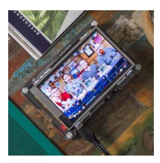
A high-resolution, high-speed 3.5" TFT display for your Raspberry Pi.
