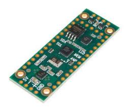
**Description:** The Teensy Prop Shield is meant for making interactive light and sound effects on small, handheld props and wearable costumes. This shield features 10DoF (Degrees of Freedom) motion sensors, a 2W audio amp, high-speed 5V buffers for driving APA102 LEDs, and an 8MB flash memory. This little board is about the size of the Teensy 3.2, just slightly longer to allow space for mounting holes and connections for power, speaker and LEDs.
