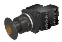
30mm BlackMax, Epoxy Coated Corrosion Resistant Complete Metal Unit Illuminated Push-Pull Operator Full Voltage, 24V AC/DC LED Lamp Mushroom Head Cap Small 1 3/4" (44.5 mm) Metal, Black with Amber Lens 3 Position Pull-Momentary/Push-Maintained 1 N.C.+1 N.C. Extra Late Break Heavy Duty Contacts, A600/P600 UL Listed, CSA Certified NEMA 1,3,3R,4,4X,12,13 & Automotive Standards
