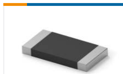
TE Part #4-2176421-1 TLRP 2512 2.0W R200 1% 25PPM 4K RL
