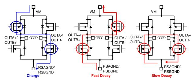
Note: Fixed value of 400 ns (design value) is prepared at the switching timing of MOSFET output to avoid any flow-through current. The equivalent circuit diagrams may be simplified or omitted for explanatory purposes.
