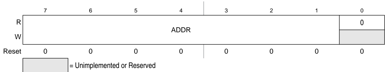
Figure 14-3. IIC Address Register (IICA)
