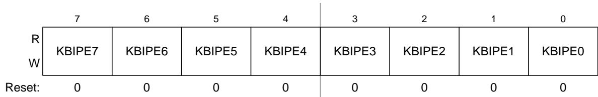
Figure 7-4. KBIx Pin Enable Register
