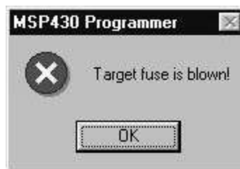
Figure 2–3. Communication Error Box for Blown Fuse
