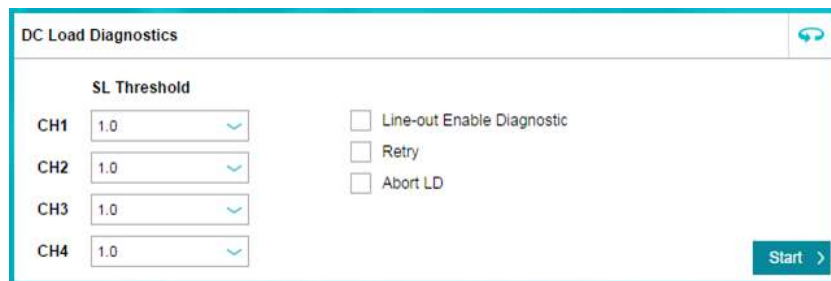
Figure 17. DC Load Diagnostics Section
