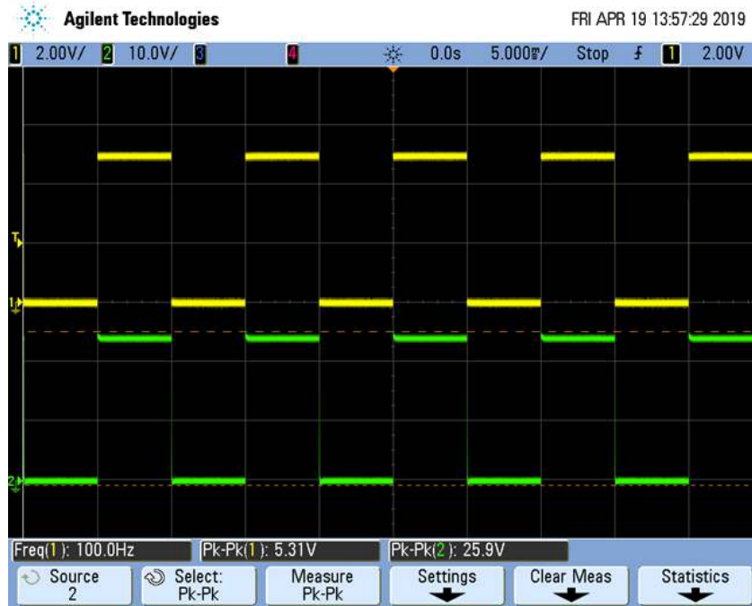
Figure 4. Oscilloscope Waveform with 100 Hz Square Wave Input
