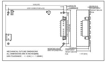
**Note** : This open frame power supply should preferably be mounted horizontally on 4 metal stand-offs having diameter not more than 6mm and height not less than 5mm
