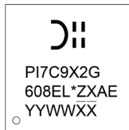
Figure 14-2 Package Bottom View
