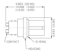
HOUSING: PBT UL94V-0, BLACK BRASS CONTACT: NUT: BRASS D-RING: EPDM, BLACK FINISH CONTACT: GOLD PLATED □VER 504" NICKEL NUT: NICKEL PLATED 60ц" ТО 100ц" OVER ALL ELECTRICAL RATED CURRENT: 4Α 250V RATED VOLTAGE: INSULATION RESISTANCE: 100 MOhms MIN. 10 m□hms MAX. CONTACT RESISTANCE: WATER PROOF: IP67 ENVIRONMENT OPERATION TEMPERATURE: -40°C TD +85°C MAX WIRE AWG: 22
