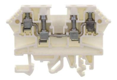
Feed-through terminal, Screw connection, Mounting type:Mounting rail TS 35/7.5 and TS 32, Rated cross-section: 4 mm<sup>2</sup>, Width: 6 mm, Colour: White
