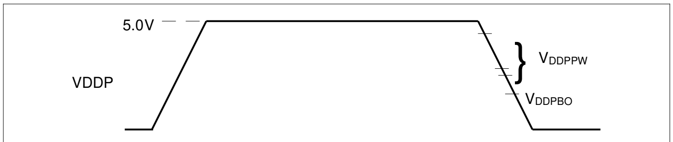
Figure 14 Supply Threshold Parameters
