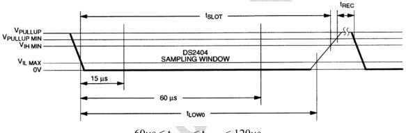
$60\mu s \leq t_{LOW0} \leq t_{SLOT} \leq 120\mu s$   $1\mu s \leq t_{REC} < \infty$
