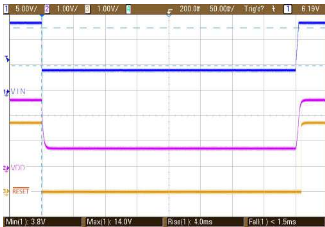
Figure 51. TPS3840-Q1 Warm-Start Test Pulse
