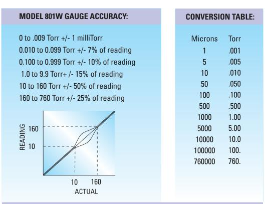
**The 801W** is a drop in replacement for the Varian 801 and other Hastings and Fredericks gauge controllers which mount in the industry standard 3 bolt pattern.
