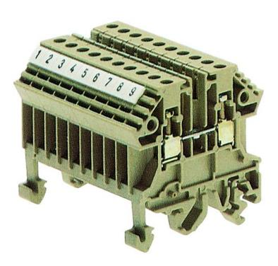
Feed-through terminal/block variant, Screw connection, Mounting type:Mounting rail TS 35/7.5 and TS 32, Rated cross-section: 2.5 mm², Colour: Beige
