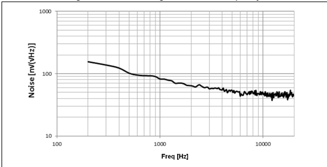
Figure 38. OPAMP voltage noise versus frequency
