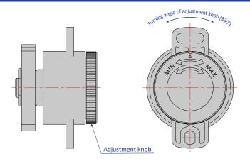
Turn the adjustment knob clockwise to increase damper torque and counterclockwise to decrease it.
