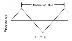
Modulation Frequency = Input Frequency/10000
