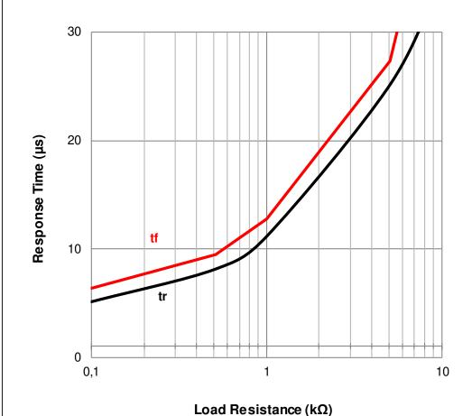
Testcondition: I<sub>C</sub>= 2mA; V<sub>CF</sub>= 2V; TA= 25°C
