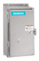
Non-reversing contactor, Size 2 1/2, Single phase full voltage, Contactor amp rating 60A, 3 wire (NO aux included), 110V 50Hz / 120V 60Hz coil, Non-combination type, Encl NEMA type 4X 304 S-Steel, Water/dust tight noncorrosive, Standard width enclosure
