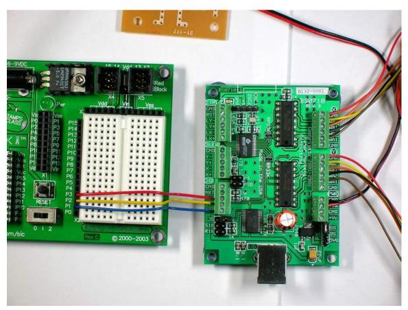
In this case, both boards were powered off of the same 12 volt power source (the BOE can support this without trouble, even though they show 9 volts as the maximum). This allows one power supply to be used to operate both the board logic and the motors themselves.
