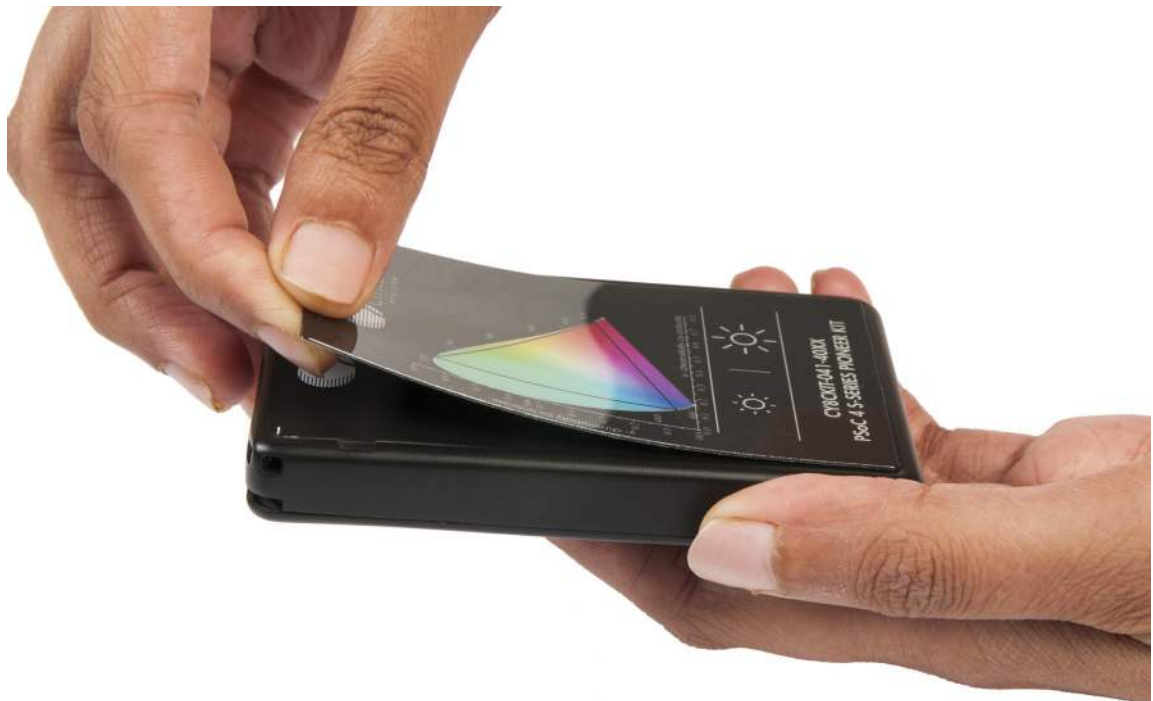
Figure 3-10. Removing the Overlay
