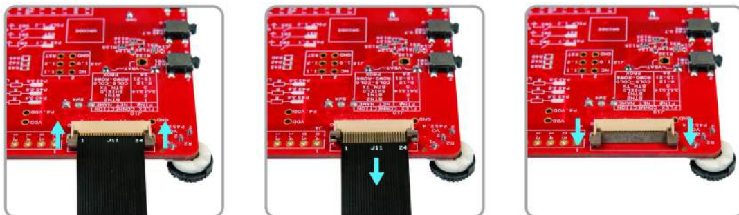
Figure 3-9. Disconnecting flex PCB from main board
