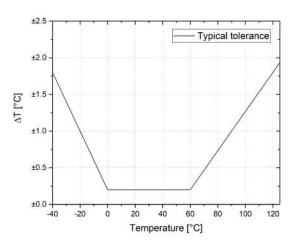
Fig. 2: Typical tolerance of the temperature measurement
