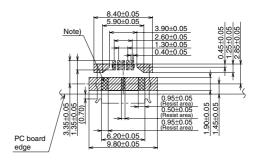
Note) : PC board pattern :: Apply resist onto the PC board pattern.
