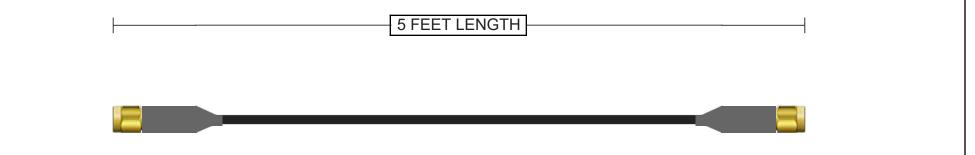
Connector A 132451 SMA Plug Straight Brass Gold + Heatshrink 50 Ohm LMR-240 Continuity/Hi-Pot Connector B 132451 SMA Plug Straight Brass Gold + Heatshrink
