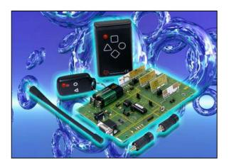
The RFEVAL2 / RFEVAL3 are hardware development platforms designed to assist the engineer design a remote telemetry application. Each project uses the advanced RF600E and RF600D Keeloq protocol and a variety of radio modules. Our aim with this Evaluation kit is to assist the engineer in designing a remote telemetry application with optimum Range.
