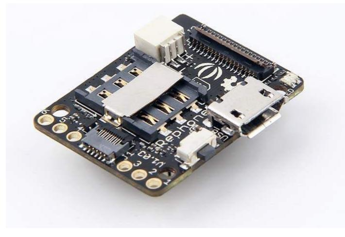
Whether making and receiving telephone calls over a radio link using external speakers and microphone or exchanging data in short distances with Bluetooth, you can do it with Xadow GSM+BLE.
