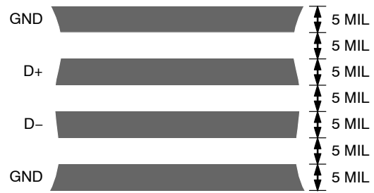
Figure 22. Typical Arrangement of Signal Tracks
