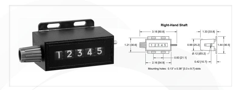
A compact, 5 figure, rotary counter, indicating 10 counts/revolution. Design and compact size make it ideally suited for office and test equipment, coin counting and other direct reading instruments.
