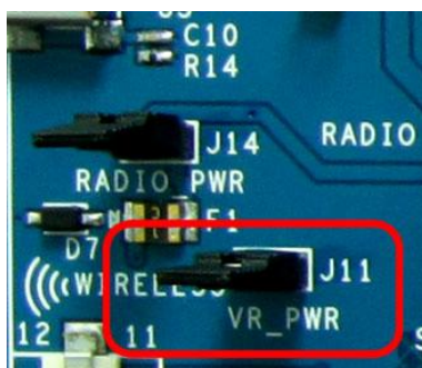
Figure 4-5: CY8CKIT-001 PSoC DVK VR_POWER Jumper
