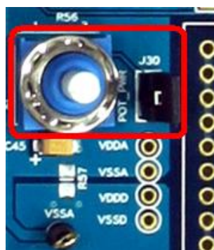
Figure 4-7: CY8CKIT-030 PSoC 3 DVK Potentiometer Power
