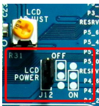
Figure 4-4: CY8CKIT-001 PSoC DVK LCD Power Jumper
