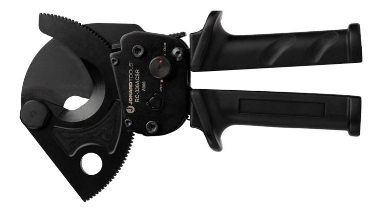
Designed for heavy-duty use, This cable cutter is designed to cut 336 MCM (170 mm<sup>2</sup>) ACSR, 400 MCM (202 mm<sup>2</sup>) copper, or 600 MCM (304 mm<sup>2</sup>) aluminum cables, and most cables up to 30mm in diameter. This cable cutter features the following:
